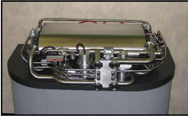
Fig. 7. Fuel processor packaging study using automotive-type components.
